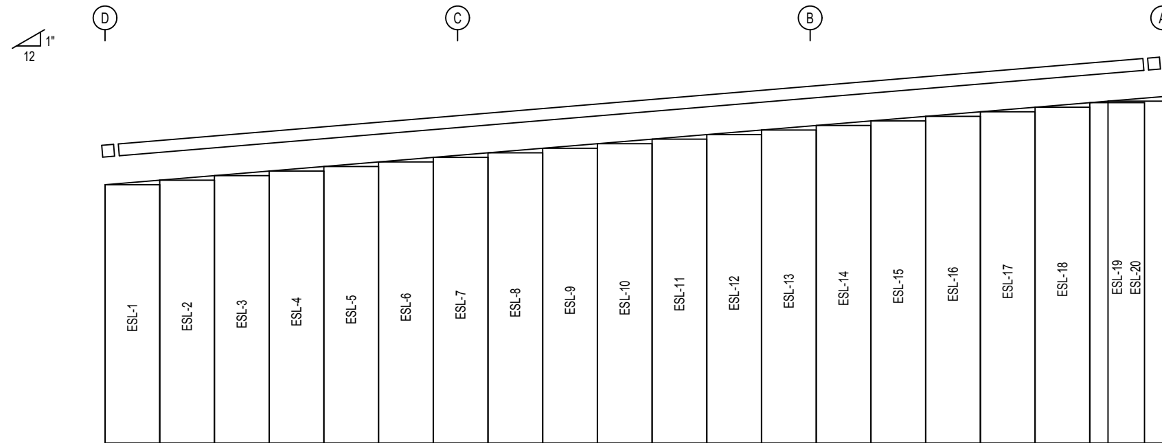
ENDWALL SHEETING & TRIM: FRAME LINE 1
